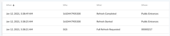
If the refresh does not start or complete, re-verify signal strength connectivity. Move the connector closer to the SGS if necessary.
